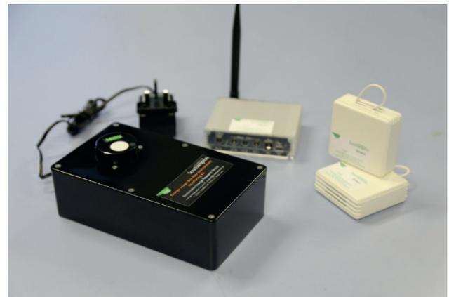
Figure 1. A monitoring kit was developed to collect temperature, energy consumption and carbon dioxide data from residential buildings in Southampton, UK.
