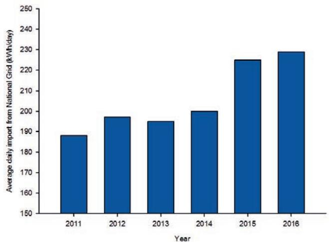
Figure 1.5. Electricity import from the national grid for the days the CHP did not run (June, July, August 2011 – 2016).
