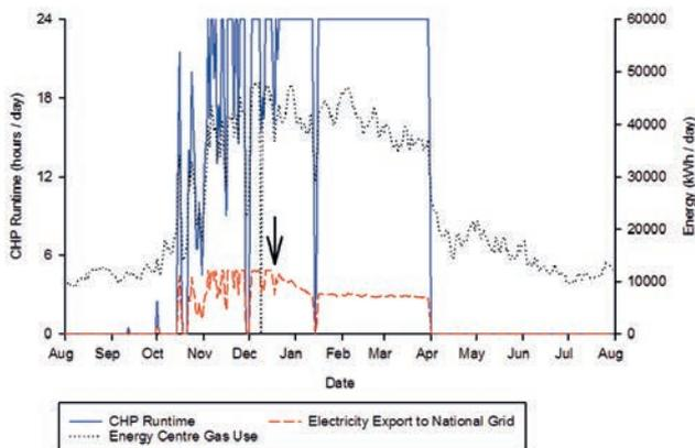
Figure 1.3. The electricity generation (red line) and the runtime (blue line) of the CHP. The arrow shows the event that led to the decrease in electricity generation.
